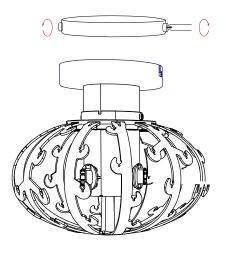
Connect the electrical connector (2) to the base located on the ceiling or wall Attach the central body (4) to the base (1) fixed to the ceiling, turn the body until it comes to a full stop and tighten the attachment screws (3) and then insert the light bulbs. Insert the bulb into the tool provided(7). Mount the bulb in the socket and press the plunger until the bulb releases.
