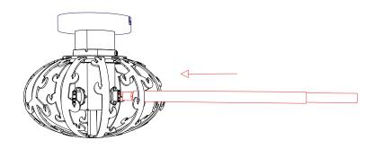
Insert the bulb into the tool provided (10). Mount the bulb in the socket and press the plunger until the bulb releases.
