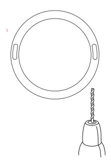
Place the base (1) on the ceiling in the desired position and make a mark on each side to indicate the diameter. Then remove it and make two holes with a Ø6 mm drill bit. And use anchors provided for attachment.
