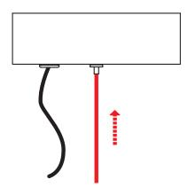
To centre the lamp, adjust the metal cord, which must remain taut with respect to the power cable. Move the cord towards the part of the lamp that is closest to the ground.
