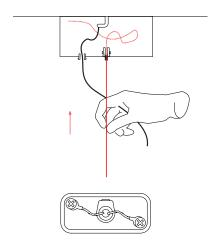
Push the metal cable (5) into the piston until the lamp reaches the desired height. If the product exceeds the desired height it can be drawn back by pressing with a finger the piston highlighted in red.
